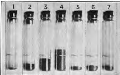
FIG. 4.—RELATIVE AMOUNTS OF DIFFERENT SIZED PARTICLES COMPOSING A SANDY SOIL.
